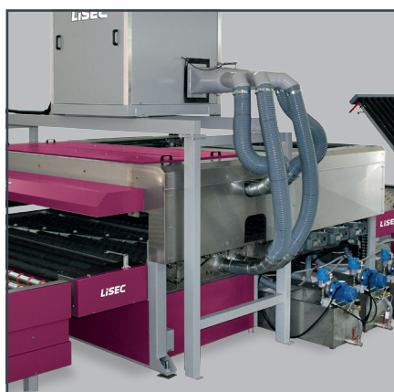
Inclined air knives for a perfect drying
