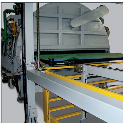
Laminating Tunnel exit, automatic tray unloading and storing into the buffer
