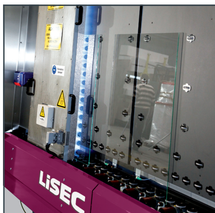
Light exposure using cold light for the chemical connection of the coating and the glass sheet
