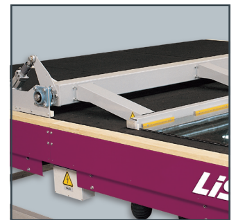
Movable stop bar for half-automatic positioning.
